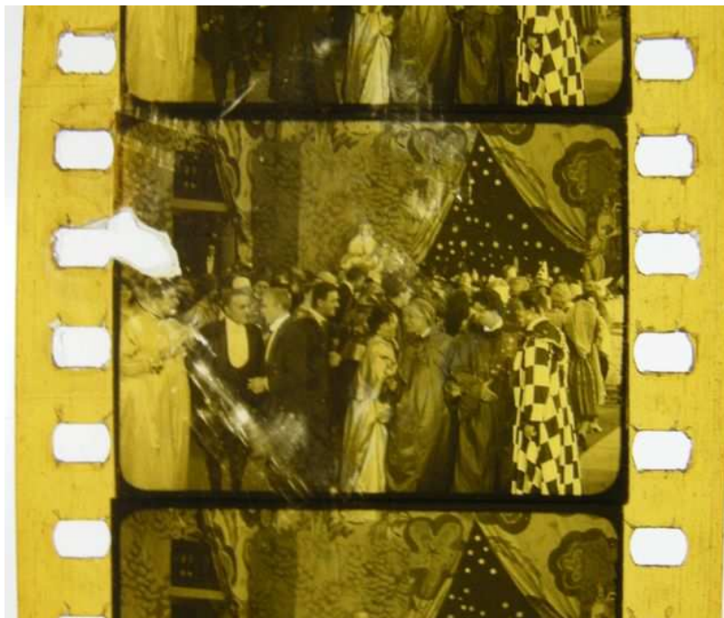
Scratching, base damage
